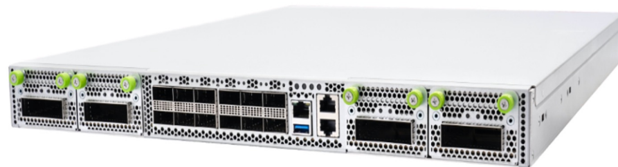
Galileo (2019) 1RU Line: 4*CFP2(100G/200G) HW: Wistron SW: Goldstone、OcNOS
