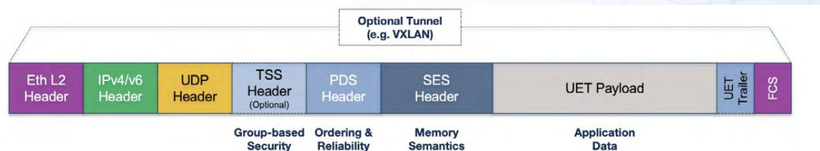
Figure 2: UET Packet Format
